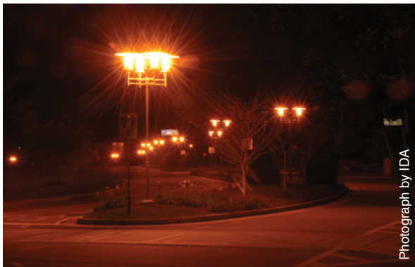
Glaring lights can actually reduce visibility. Here the brightest most visible objects in the area are the lighting fixtures, not the roadways, walkways or parking areas which a driver or pedestrian would expect to be lighted. Atlanta, Georgia.
